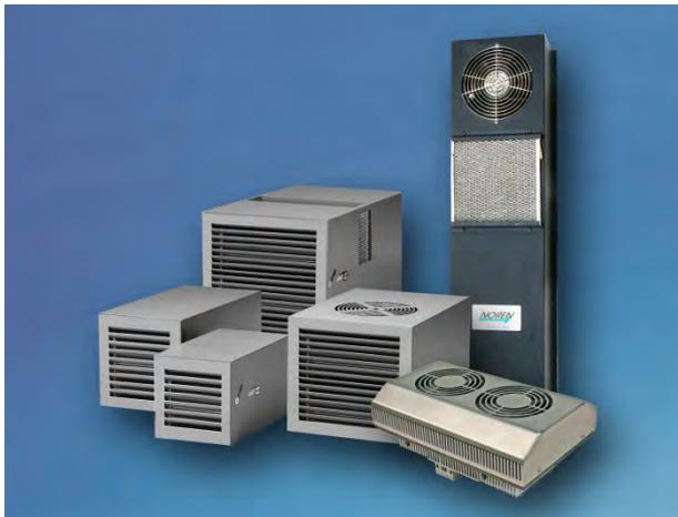
Thermoelectric recirculating chillers are available from 150W to 950W of cooling capacity and offer precise temperature control to  $\pm 0.05^{\circ}\text{C}$ . These chillers feature whisper-quiet operation, vibration-free operation, world wide power compatibility and a high efficiency variable voltage source that consumes energy only when needed.
